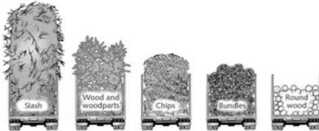
Figure 2. Volumes of different kind of forest products compared per full truck load 3
