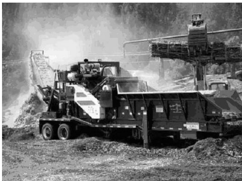
Figure 4. Mobile horizontal grinder in the US processing bundled slash 6
