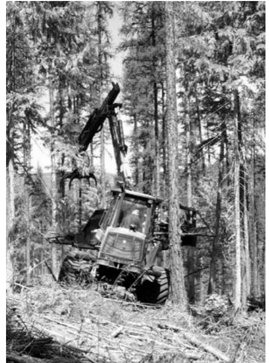
Figure 6. Bundler operating in a stand after a thinning 7
